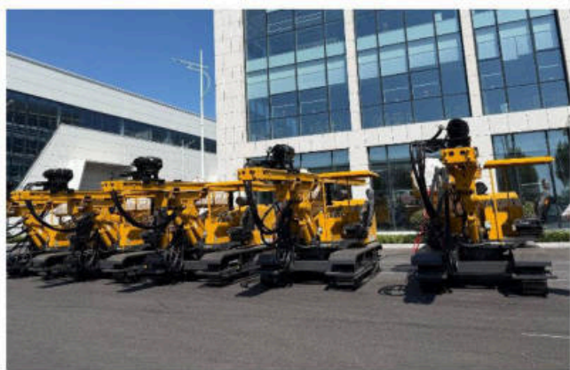
CRAWLER PILE DRIVERS, THE FOUNDATION PLANT FOR GROUND-MOUNT ARRAYS
